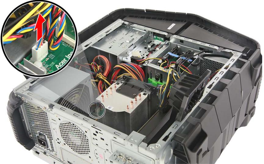
3. Use a long screw driver to loosen the four captive screws securing the thermal module to the mainboard.
