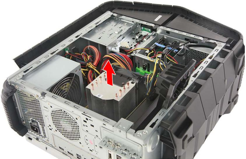
5. Release the cables from the cable clip securing them to the HDD bracket.
