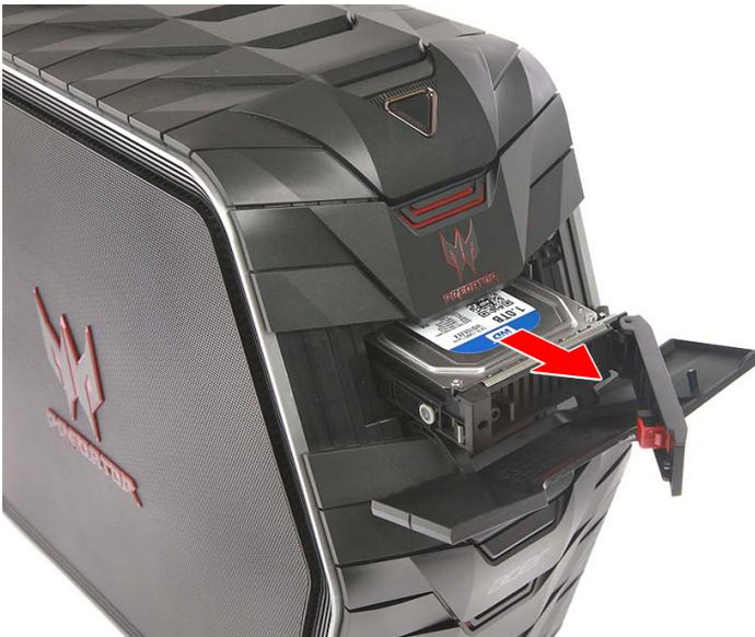
6. Pull both sides of the HDD carrier (1) then remove the hard drive (2).
