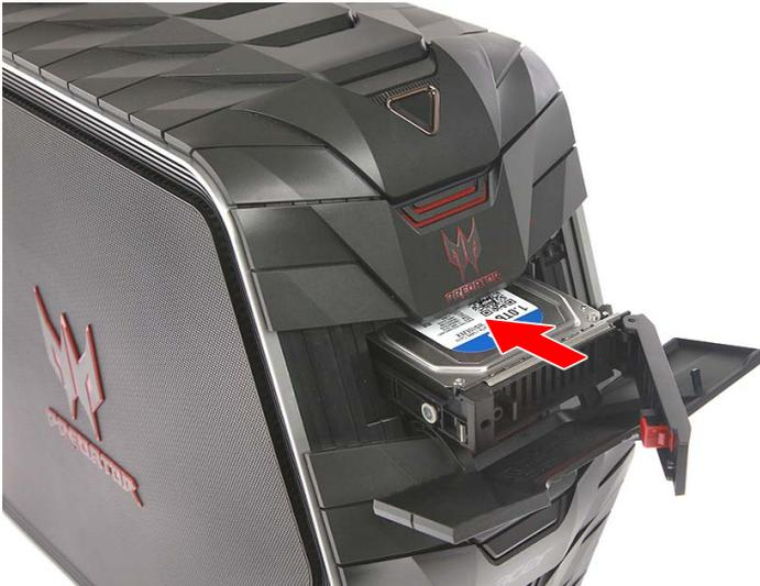
4. Push the HDD carrier lever until it latches into place.
