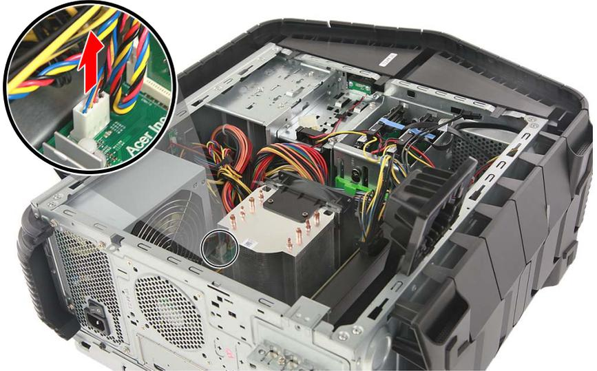
3. Use a long screw driver to loosen the four captive screws securing the thermal module to the mainboard.
